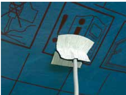
7. Remove the remaining backing strips and press together
