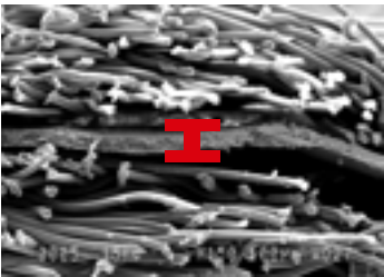
Standard multilayer Membrane: 30 microns (internally measured)
