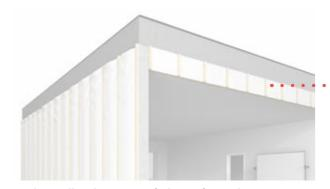
High windloads causing failure of membranes Loose membranes causing obstruction of needed ventilation behind facade boards.
