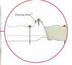
Galvanised steel strip allows sidelaps to be secured and reliable fixing with standard fasteners.
