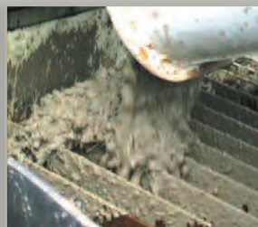
2. Fibres mix perfectly with concrete
