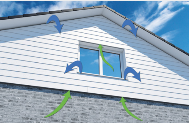
→ Green: Air inlets → Blue: Air Outlets
